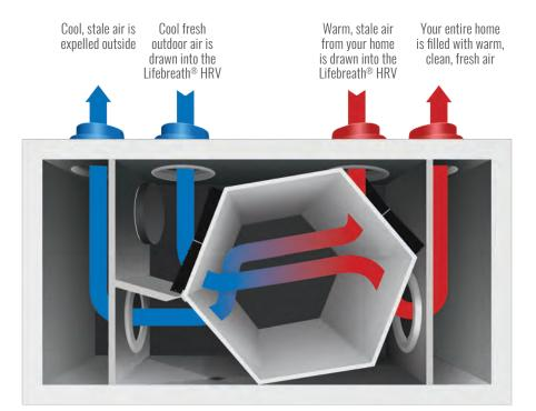
Heat from the indoor air is transferred via the unit's aluminum core to the incoming fresh air stream.
